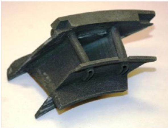
High pressure turbine nozzle segments: cooled doublet vane sections.
