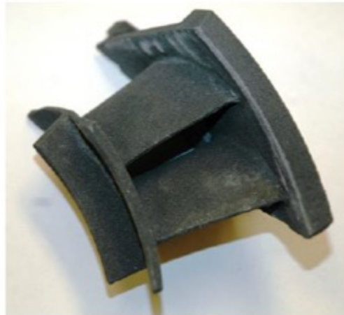
High pressure turbine nozzle segments: cooled doublet vane sections.
