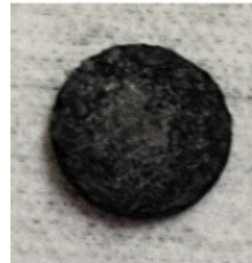
Laser cut prepregs used for composite processing
