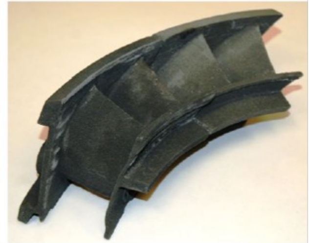
High pressure turbine nozzle segments: cooled doublet vane sections.
